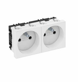
Socket with earthing pin, double 0°, with increased touch protection, with screwless terminals, 2-pin, 16 A, 250 V~, with connection terminals to IEC 60884-1.
