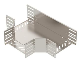
T piece for the creation of a horizontal branch, fitting for lock and screw-on cable trays of side height 110 mm. Screwless mounting with double clamps or screw connection with FRS truss-head screws and M6 combination nuts. Can be used indoors and outdoors. Fastening material must be ordered separately.
