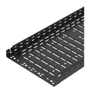
Cable tray with integrated quick-fastening system. Strip-galvanised surface, visible areas powder-coated in jet black (RAL 9005). Continuous side perforations of 7 x 20 mm for the installation of additional connection and mounting components. With 11 mm perforation in the base for direct threaded rod suspension. Usable length 3,000 mm.
