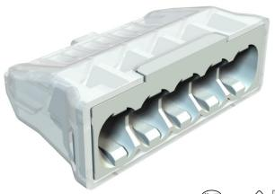
Screwless terminal to connect single-strand cables. Nominal cross-section 2.5  $\div~mm^2$ Rated voltage450 V Rated current24 A 5 x 0.5 mm<sup>2</sup> to 2.5 mm<sup>2</sup> single-wire cable
