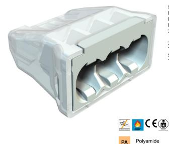
Screwless terminal to connect single-strand cables. Nominal cross-section0.5 ÷ 2.5 mm<sup>2</sup> Rated voltage450 V Rated current24 A 3 x 0.5 mm<sup>2</sup> to 2.5 mm<sup>2</sup> single-wire conductors
