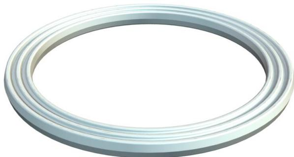
Connection thread sealing ring, suitable for all plastic cable glands, with metric thread according to DIN EN 60423 or ISO 68. The internal diameters of the sealing rings are designed in such a way that they can be pre-mounted in a captive manner.
